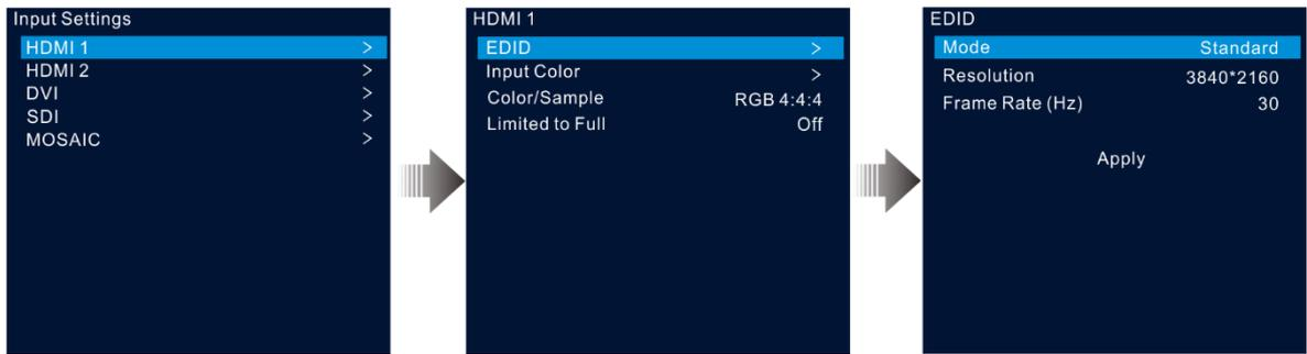
Step 8 Rotate the knob to select **Apply** and press the knob to complete the standard resolution settings.
