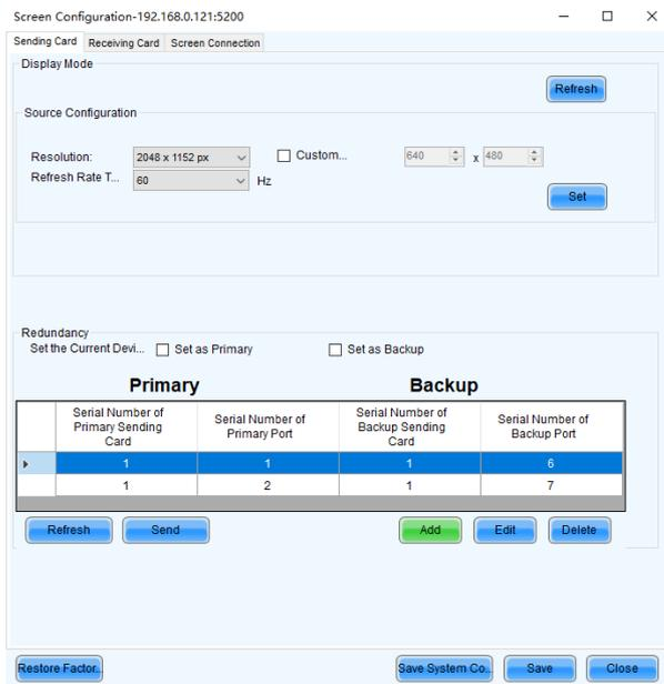
Step 8 Repeat Step 6 and Step 7 to complete the backup settings for other Ethernet ports.
