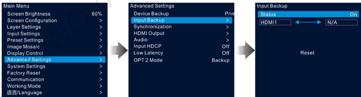
Step 2 Rotate the knob to select **Status** and press the knob to confirm. Rotate the knob again to select **On** and press the knob to confirm.
