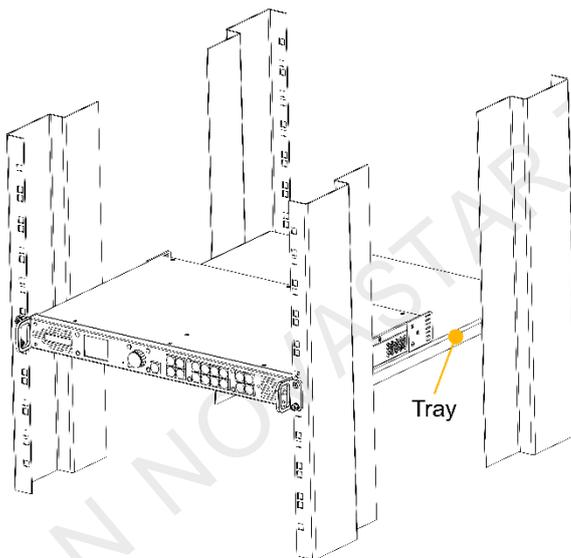
1. Elevated Operating Ambient - If installed in a closed or multi-unit rack assembly, the operating ambient temperature of the rack environment may be greater than room ambient. Therefore, consideration should be given to installing the equipment in an environment compatible with the maximum ambient temperature (T<sub>ma</sub>) specified by the manufacturer.
