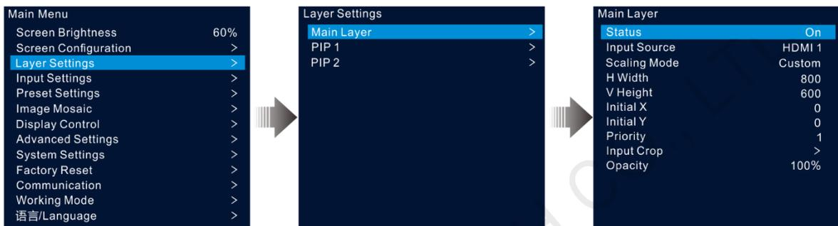
Step 4 Select **Status** and press the knob to confirm. Rotate the knob again to select **On** and press the knob to confirm.
