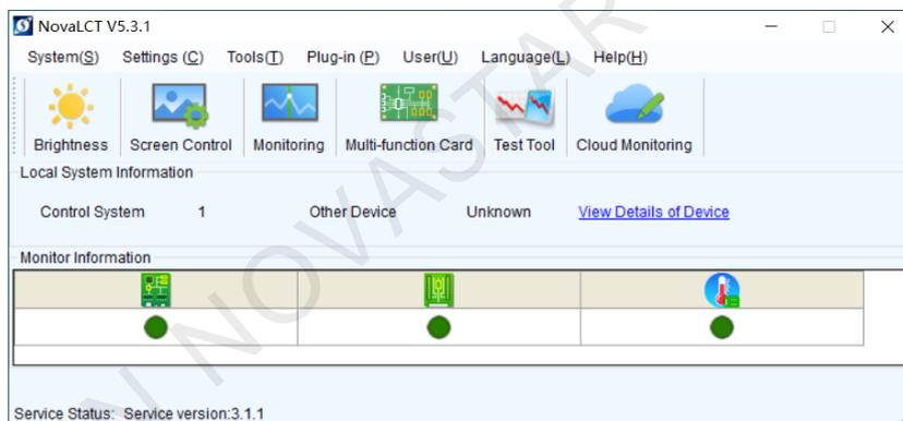
Step 2 Go to **Tools > Controller Cabinet Configuration File Import** to enter the controller cabinet configuration file importing page.
